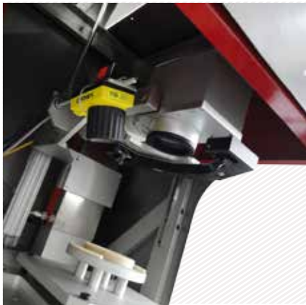
XL-Box marking station with deported reading system
