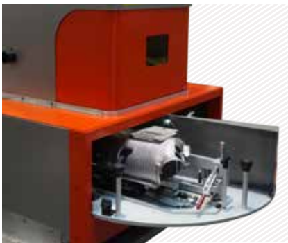
Laser station equipped with a turntable
